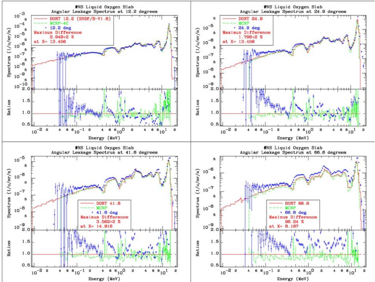
**Fig. 3:** Measured spectra from the FNS Liquid Oxygen Benchmark, compared to the calculated spectra obtained using the DORT and MCNP4C codes with multigroup and point-wise ENDF/B-VI.8 cross-sections, respectively.
